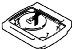
**Step 2:** Remove another 4 screws on the circuit board.
