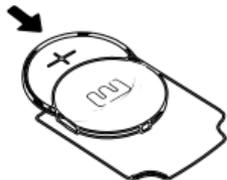
**Step 4:** Insert the new battery, keeping the "+" post facing
