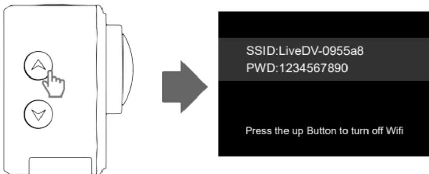
■ **Turn off mobile data and connect the camera and smartphone via a WLAN network.**
